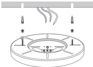
Method b: Check and confirm the installation position, connect the cables into wiring terminals, and then fix the base on the ceiling by metric screws properly and securely.
