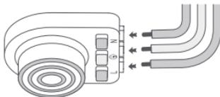
Connect cables into Neutral wire, grounding wire and live wire marked by N,  $\oplus$  and L. Respectively (Please tap the red button on the terminals before withdrawing cables).
