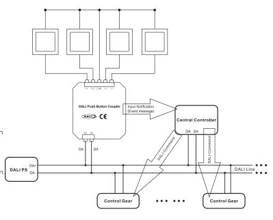
The SYMPHO DALI Push Button Coupler supports 4 instances (1 - 4) of type 1 (IEC62386-301, Input Devices - Push Button) which are assigned to the 4 button inputs.
